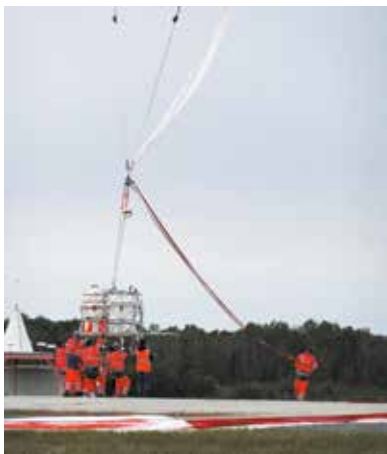
The gondola is hoisted into position.
