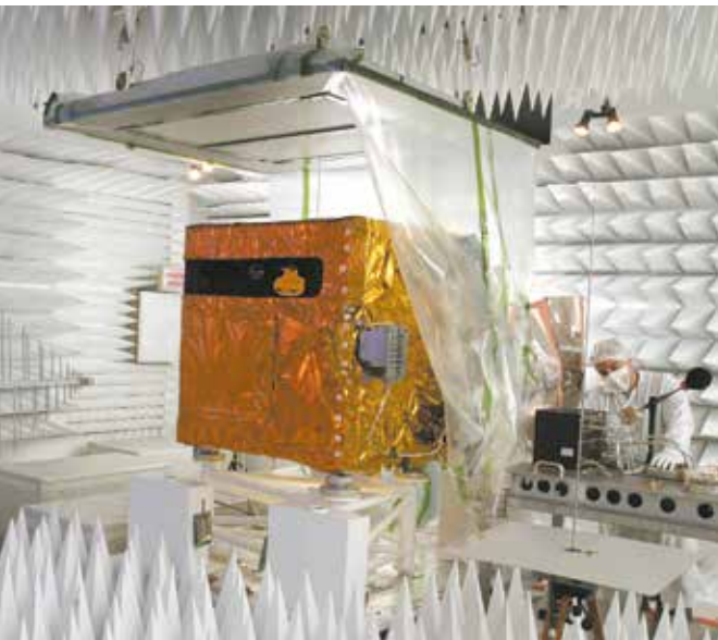
The instrument undergoes electromagnetic compatibility testing in an anechoic chamber, the SWIM instrument.
